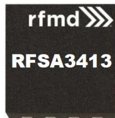
16 Pad 3.0 x 3.0 x 0.85 mm QFN Package
